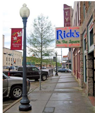
Acorn lights around the square are the right height for pedestrians but rather widely spaced for optimum light distribution.
