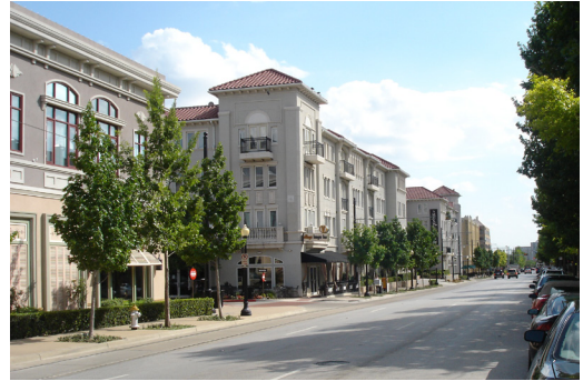
New development should be close to sidewalks and have on-street or rear parking.
